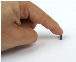
the pins. If you need to take the chip out, pry it gently with a small screwdriver, alternately prying both ends of the chip.
