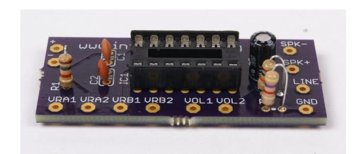
Mount the 130  $\rm Ohm$  1 watt resistor in the holes marked Vol1 and Vol2  $\rm This$  resistor will limit the power going to the speaker, and prevent the IC chip from being damaged.
