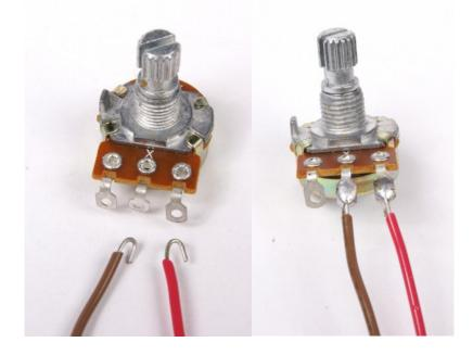
Solder the pair of wires from one of the 500 kohm potentiometers to the holes marked **VRA1 and VRA2.** It doesn't matter which wire goes in which hole.
