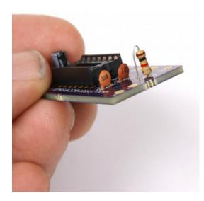
Solder the 1kOhm(brown black red) resistor in the spot marked R1. Make sure you don't get it mixed up with the 10 kOhm resistor- red and orange can look very similar! In a similar fashion mount the 10 kohm (brown black orange) in the spot marked R2, and the 4.7 kohm resistor in the spot marked R3. Your board should now look like this:
