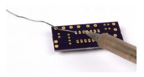
Solder each pin of the socket to the circuit board. It's a good idea to flip the board over and check that it's straight after soldering one pin, then go ahead and solder the rest. Take care that adjacent pins don't get shorted together by blobs of solder, and that you've soldered all 14 pins.
