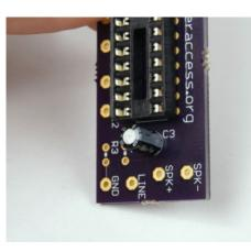
C3, the 10µF electrolytic capacitor has to be installed the correct way around. Make sure the long lead goes through the hole marked "+" in the circle marked C3. The negative (-) side should be marked on the body of the capacitor.
