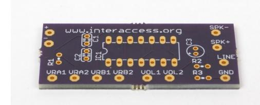
First, examine the printed circuit board. We will install components on the top side, which is the side with the printing on it.
